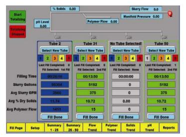
The SmartFeed™ system monitors slurry characteristics, such as density, percent dry solids, flow, pH, pressure and polymer induction shear velocity, and recalculates the dose rate every 15 seconds based on these changing parameters — maintaining optimum performance of the Geotube® containers and polymer.
