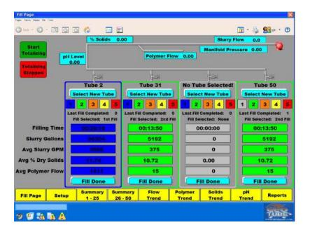
The SmartFeed™ system provides full reporting of dewatering performance for each Geotube® container in the project—including filling time, gallons of slurry pumped, average gpm, average percent dry solids and average polymer flow.
