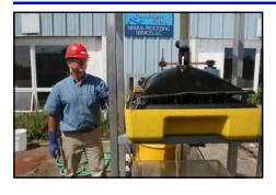
First phase fill: Operate fill pump until pressure gauge located on pump discharge achieves discharge pressure of Geotube circumference. 30' circ 2.6 psi; 45' circ 3.0 psi; 80' circ 3.5 psi.
