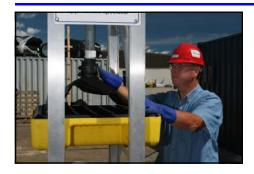
Insert 2" hose supplied with test unit in to sample storage container using test stand pump for transfer slurry to mix tank. *Place Valve 1 handle in suction position*
